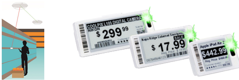
Figure 1: The Pricer Electronic Shelf Label system replaces paper price labels with digital screens connected to the network. In the right image the IR transmitters and the controllable green LEDs can be seen on each price label.
