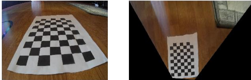
(a) Raw image from robot camera feed. Chessboard pattern is used to find perspective warp (homography) from ground to image plane. (b) Undistorted and perspective wrapped image from raw image in (a). A top-down view of the calibrated plane is achieved.
